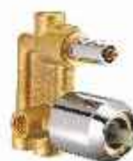
3 Inlet Single Lever Concealed Diverter Body consisting of 45mm Cartridge with Tip Ton and Cartridge Sleeve (Excluding operating lever, wall flange and tip ton handle)
