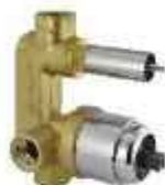
High Flow Single Lever Concealed Diverter Body consisting of 40mm Cartridge with Tip Ton and Cartridge Sleeve (Excluding operating lever, wall flange and tip ton handle)
